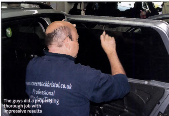
Once in the workshop the trim was removed and the film carefully applied
